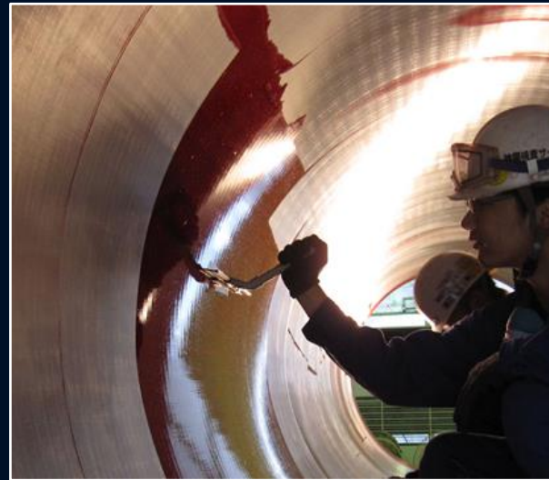
Alternative test method to penetrant test Object: steel pipe
