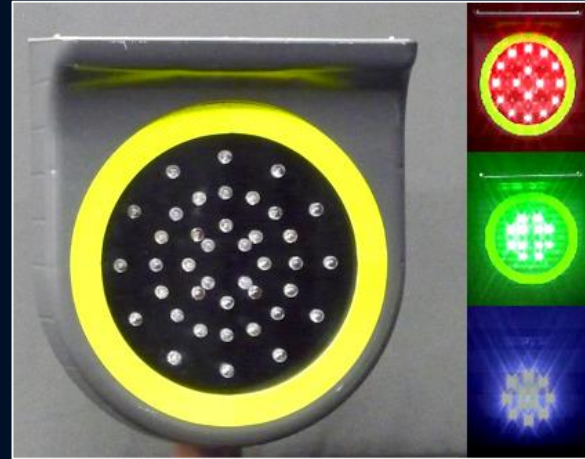
Utilization of luminance (after glow) by application to delineator resin cover
